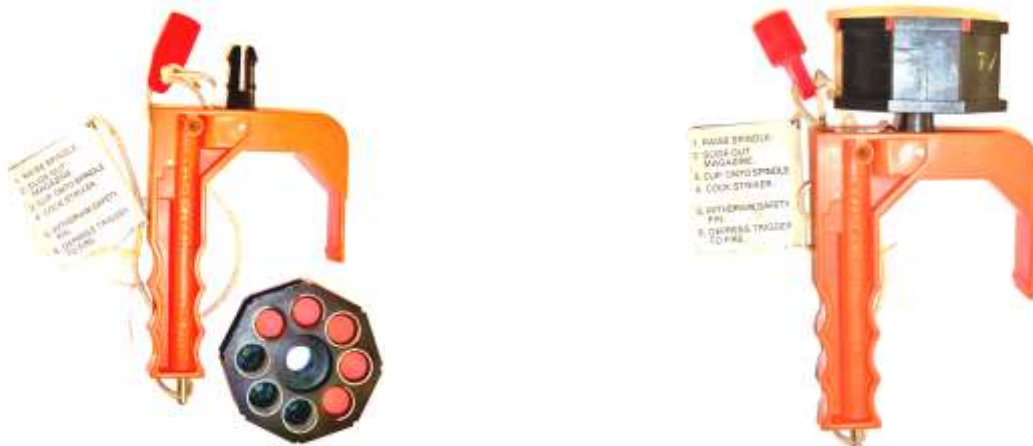
Pic 7 Dial a star distress signal device (lab exhibit 66517)
