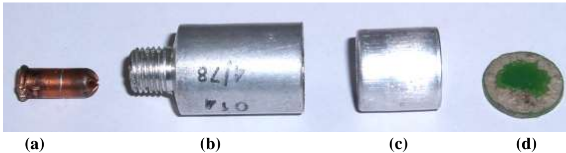
Pic 12 Mini flare components: .22 blank cartridge (a), barrel and chamber (b), flare in its container (c), over card seal (d)
